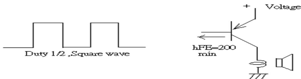
The base current  $I_b$  should high enough so that it saturates the collector current of the transistor with the CB load.
